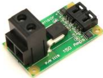
■ Figure 195: Analogue current meter module 0-50 A
