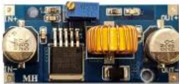
■ Figure 288: Variable voltage step-down converter module
