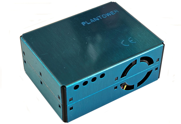
■ Figure 224: PMS5003 laser sensor for PM1.0, PM2.5 and PM10 - airduct fan side
