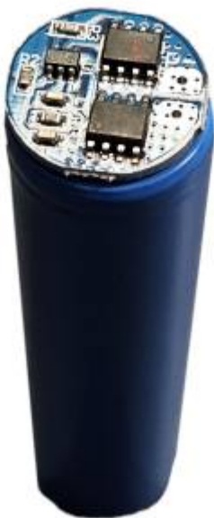
■ Figure 276: 18650 cell with protection module applied
