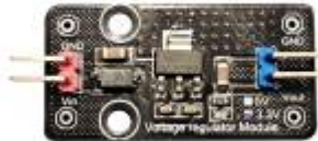
■ Figure 287: Fixed voltage step down converter module
