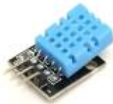
■ Figure 217: Temperature and humidity sensor module
