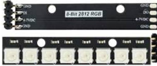
Figure 236: WS2812 8 smart LEDs stripe
