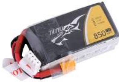
■ Figure 271: Sample 850mAh 3S LiPo battery pack
