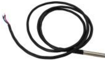
■ Figure 215: DS18B20 temperature sensor, waterproof version
