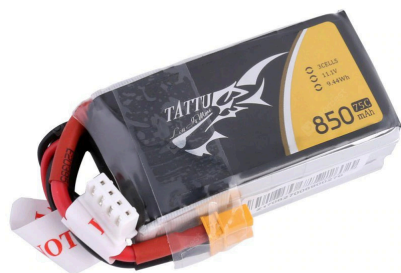
■ Figure 272: Sample 850mAh 3S LiPo battery pack
