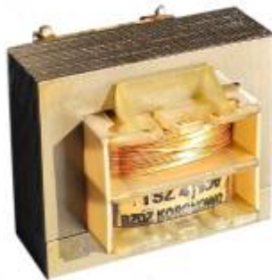
■ Figure 281: Sample high to low voltage transformer
