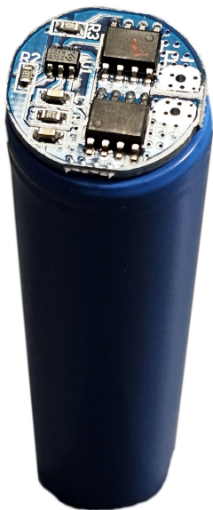
■ Figure 277: 18650 cell with protection module applied
