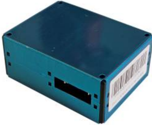
Figure 224: PMS5003 laser sensor for PM1.0, PM2.5 and PM10 - connector side
