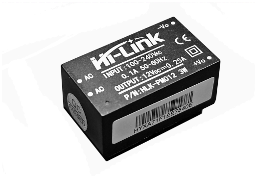
Figure 285: Sample AC to DC converter with voltage stabilised output
